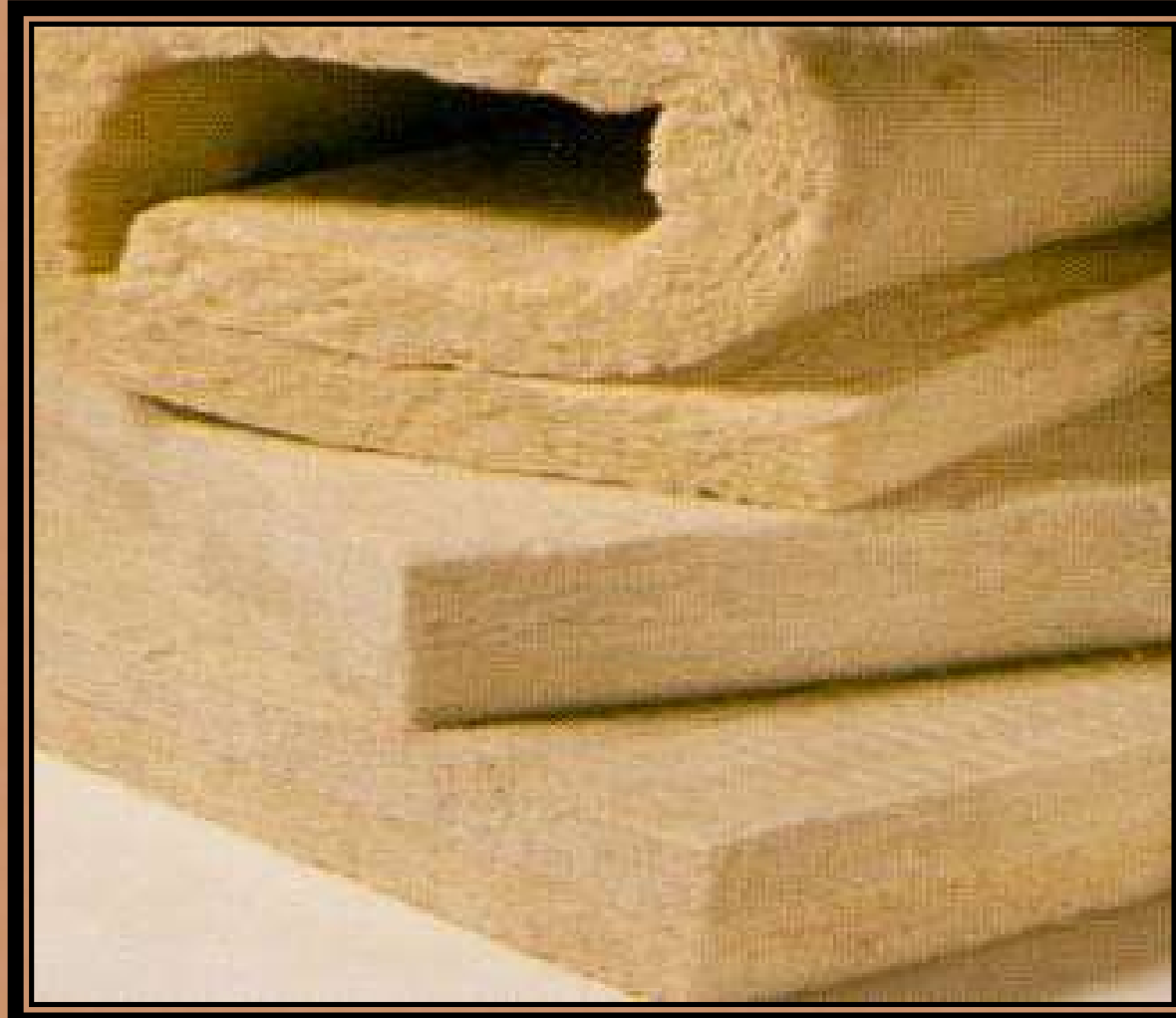
Impregnirane meke ploče ( \gamma = 35\text{kg/m}^3 )
